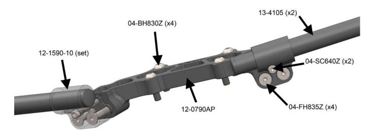
5. Use the four 04-BH830Z mounting bolts to secure the Woodcraft adapter plate to the OEM handlebar uprights as shown above.
