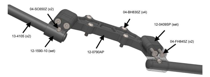
16. Use the four 04-BH830Z mounting bolts to secure the Woodcraft adapter plate to the OEM handlebar uprights as shown above.
